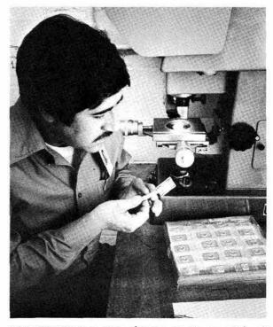
INSPECTING incoming shipments, Demmy Edwell (1411) examines microelectronics packages with an optical comparator. The work is part of a new QA inspection service.
